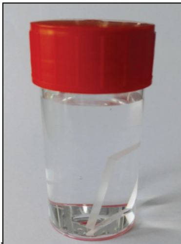
Fig. 2. The plasma activated PET plate immersed in the chitosan solution.
