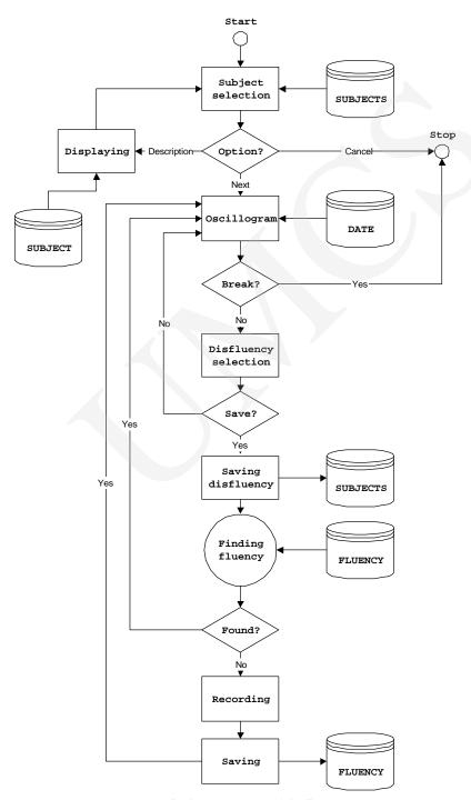
Fig. 2. Diagnosis module diagram
