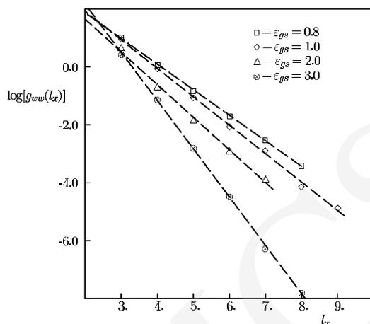
Fig. 3. Plots of the logarithm of the wall - wall energy versus the wall - wall separation for the striped phases with heavy walls, obtained for the systems with  $s^* = 1.27$ ,  $V_b = 1.0$  and different  $e_{gs}^*$  (shown in the figure)
