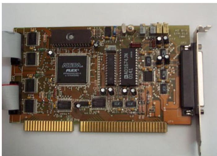
Fig. 3. The analog-digital card ADC615
