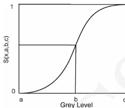
Fig. 1. Graph of the standard S-function, b=(a+c)/2 , bandwidth \Delta b=b-a=c-b and k=2
