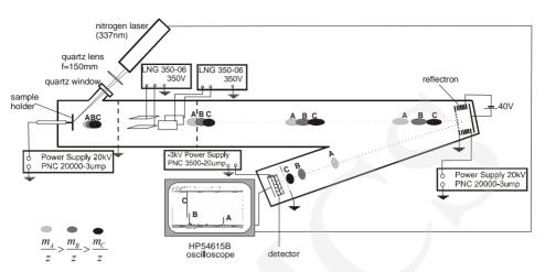
Fig. 1. The TOF MS scheme and the idea of ions formation and separation
