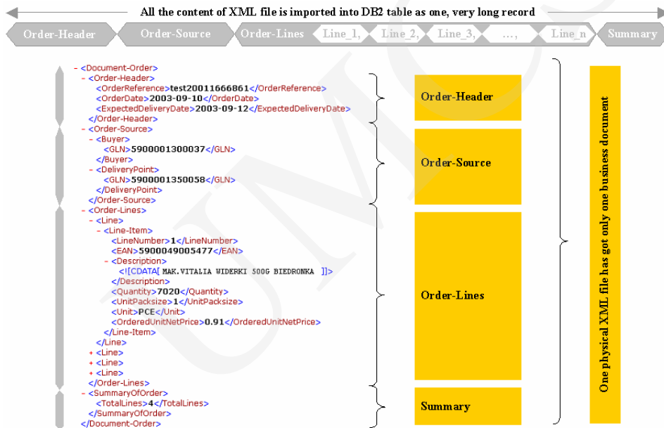
Fig. 3. The logical structure of the XML file example - provided by firm B
