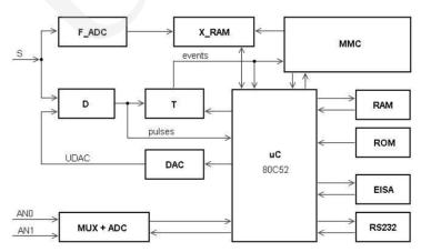
Fig. 2. Block diagram of random events recorder
