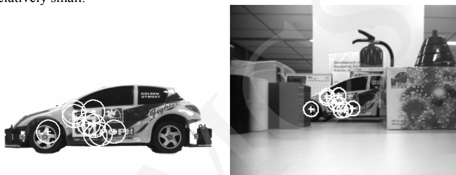
Fig. 8. Interest points automatically matched in a model image and a camera-captured view
