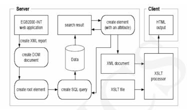
Fig. 4. Architecture of XML reporting mechanism for the internet system with HTML output
