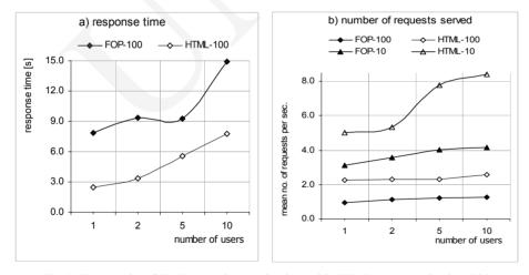
Fig. 7. Test results of XML reporting mechanism with HTML output and using FOP
