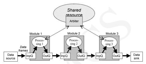
Fig. 1. Flow of data in a three-module pipeline with a shared resource
