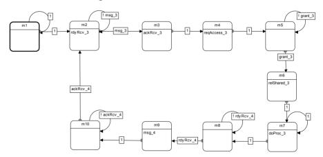
Fig. 3. CSM model of Subsystem 3 (reduced product of six components of module #3)
