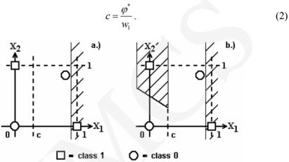
Fig. 2. Subsequent stages of an evolution of decision space for single Sigma-if neuron with two neuronal inputs during signals aggregation, a) division into two problems and solving of a linear problem, b) connection of decision spaces of the first and second stages
