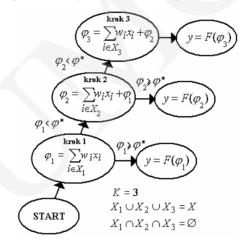
Fig. 1. The sample process of a three-step input signals' aggregation in the Sigma-if neuron
