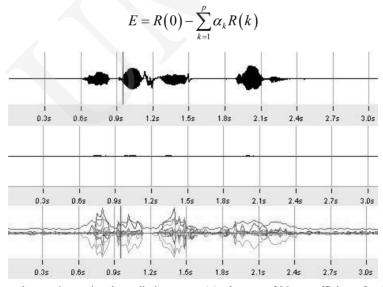
Fig. 1. From the top: input signal, prediction error e(n), changes of 20  $\alpha$  coefficients for the sample "mleko jest zdrowe". Window witdh – 29 ms. The screenshot comes from a program created by the authors of this paper
