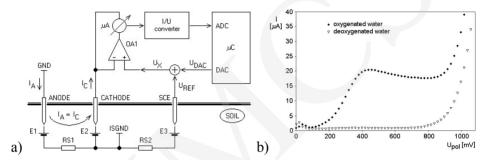
Fig. 1. The measuring circuit for determination of oxygen stream density in soil (a) and typical characteristics I = f(U) for two different oxygenation levels in deionization water (b) [2]
