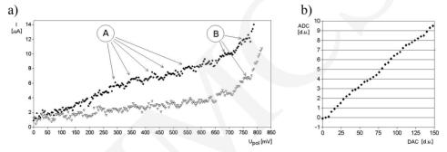
Fig. 4. Voltammetric curves with the errors resulting from measurement equipment (a) and diagram of DAC converter calibration curve fragment (b)
