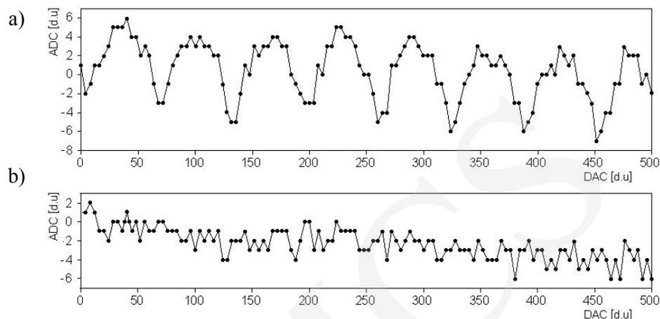
Fig. 5. DAC converter testing curves obtained from direct measurement without software correction (a) and after introduction of software correction (b). The vertical axis represent the output error generated by DAC converter
