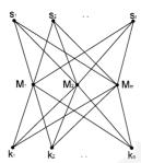
The degree of cohesion of the graph equals d = |E| - |V| + 1 = rm + nm - r - m + 1 = (r + n - 1)(m - 1). If we compare this topology with the previous one (in the previous topology m = 1 and d = 0), the degree of reliability increases m - 1 times for this SK. The algebraical notation for this topology:
