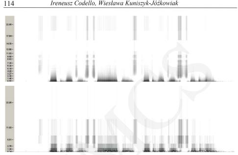
Fig. 15. Spectrum comparison of 3-second utterance "Sto dwadzieścia jeden, sto dwadzieścia dwa". From the top: LPC, FFT, CWT, DWT. In the case of DWT and CWT we used Daubechies 2 wavelet
