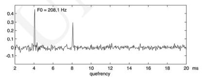
Fig. 2. F0 frequency estimation by cepstrum of speech signal
