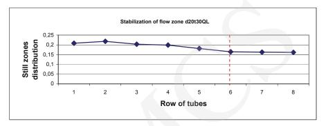
Fig. 6. Distribution of still zones area in the shell-side for square in-line arrangement  $V_L=0.42~m/s,\ V_G=0.69~m/s$
