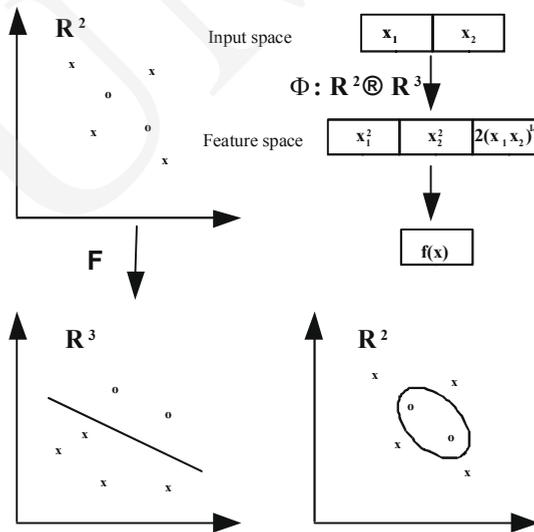
Fig. 2. Example of data separable by an elliptic curve in  $\mathfrak{R}^2$ , but linearly separable in the feature space  $\mathfrak{R}^3$ . The mapping to transforms  $(x_1, x_2) \rightarrow (x_1^2, x_2^2, \sqrt{2}x_1x_2)$ .
