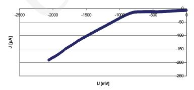
Fig. 1. Voltammetric curve with the quasiplateau interval
