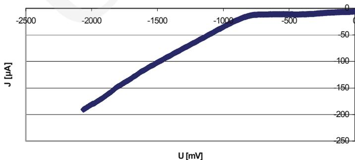
Fig. 2. Voltammetric curve with the quasiplateau interval
