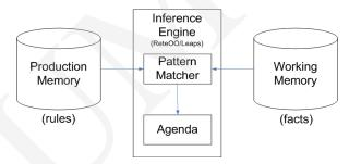
Fig.. 1. The structure of JBossRules rule engine
