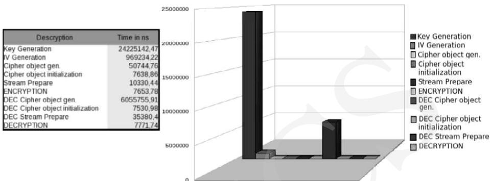
Fig. 9. Time consumption of the RSA algorithm
