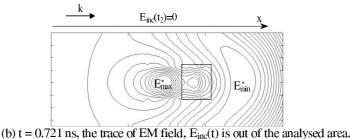
Fig. 5. Some snapshots of the propagated electromagnetic wave  $E_z(t)$  (the increment  $\Delta E_z$  of the isolevels is 0.0625 V/m)
