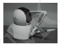
Fig. 8. The PHANTOM Omni® haptic device.
