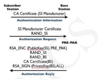
Fig. 5. Station and network authentication process in PKMv2.
