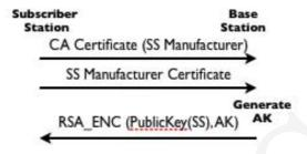
Fig. 4. Station Authentication Process.
