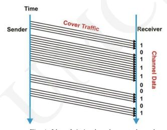
Fig. 4. Idea of timing based covert channels.
