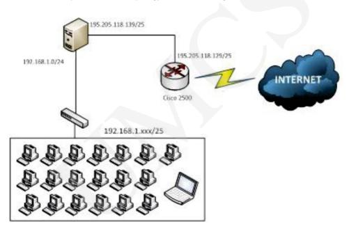
Fig. 1. Analyzed network architecture model.
