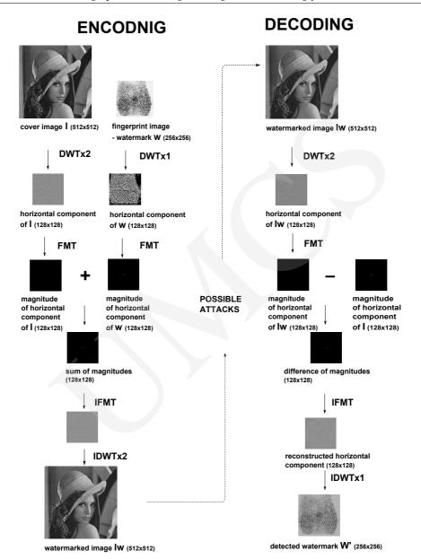
Fig. 2. Watermarking scheme, based on [11]
