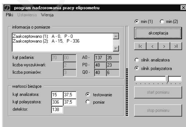
Fig. 4. Ellipsometer operation management program – graphical interface
