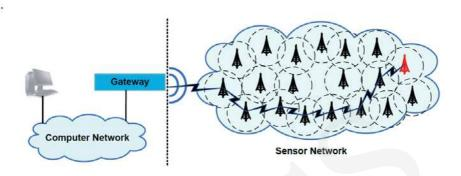
Fig. 1. The wireless sensor network architecture.
