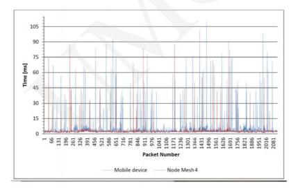
Fig. 6. Delay for packet size 56 Bytes.
