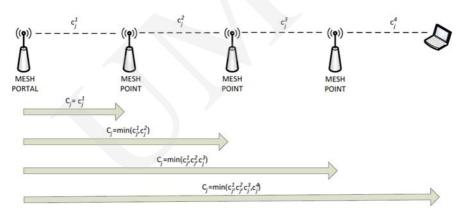
Fig. 2. Throughput in mesh networks.
