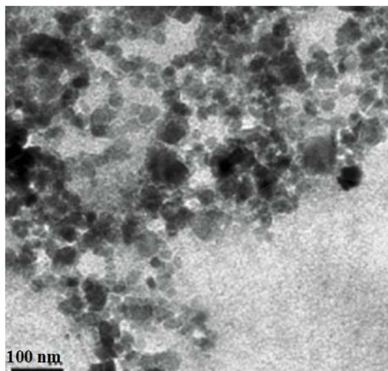
Fig.1. Large area TEM image of Fe<sub>2</sub>O<sub>3</sub> nanoparticles.
