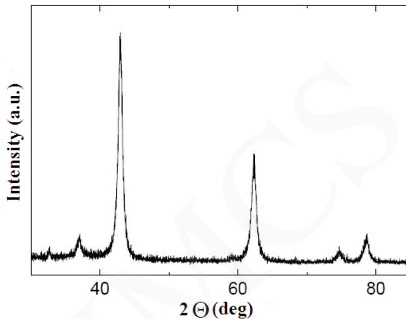
Fig. 1. X-ray diffraction pattern of nano-silicon dioxide particles.
