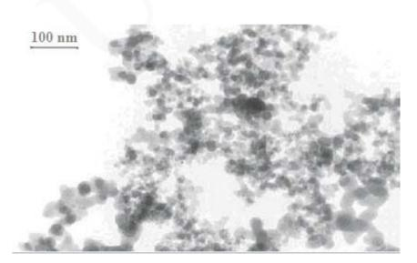
Fig. 2. Large area TEM image of Sio<sub>2</sub> nano-particles.
