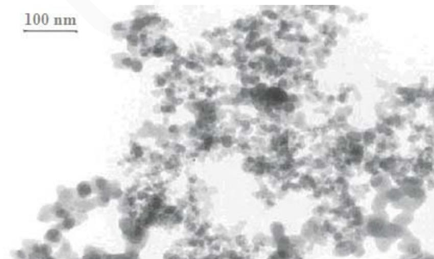
Fig. 2. Large area TEM image of SiO<sub>2</sub> nano-particles.
