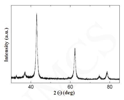
Fig. 1. X-ray diffraction pattern of nano-silicon dioxide particles.
